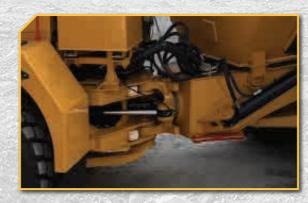
• **MULTI-ANGLE ARTICULATED FRAME** The articulated joint in the POWERPLUS PAD450Z is a robust structure connecting front and rear chassis. It allows 3-dimentional, multi-angle movement and power transmission at the same time, thus offering superb maneuverability on rough terrains.
